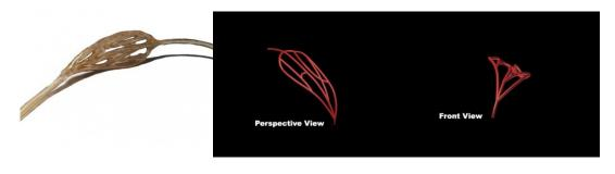
**Complex Blood Vessels** for R&D is a feature that can be implemented to any location of the brain or simply submerged in a brain mimicking material used to fill the skull or head phantom. The vessel network shown on the image is made out of our proprietary blood vessel mimicking material with realistic acoustical and MRI properties.
