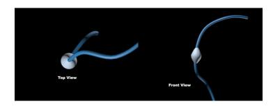
**Aneurysm** for R&D is an example of a feature that can be implemented to any location in the brain and/or blood vessels. The features shown on the image is made out of our proprietary blood vessel mimicking material with realistic acoustical and MRI properties.
