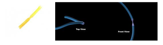
**Stenosis** for R&D is an example of a feature that can be implemented to any location in the brain and/or blood vessels. The features shown on the image is made out of our proprietary blood vessel mimicking material with realistic **acoustical and MRI properties**.
