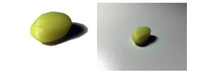
Tumor for R&D is a perfect example of a feature that can be implemented to any location of the brain or simply submerged in a brain mimicking material used to fill the skull or head phantom. The features shown on the images are made out of homogenous tissue-mimicking material with realistic acoustical and MRI properties.
