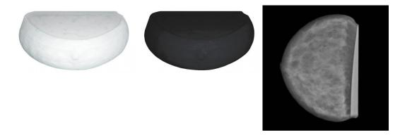
Breast phantom with adipose and glandular tissue. This breast phantom was developed to simulate breast imaging in mammography and tomosynthesis.
