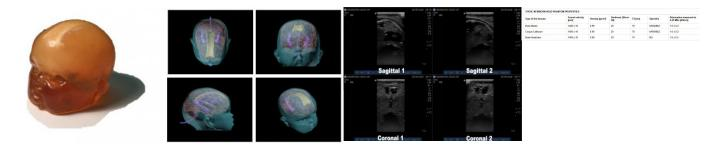
Anatomically correct phantom of a newborn's head. It was designed based on the average head of a newborn baby. Made of realistic tissue mimics, suitable for ultrasound maging.
