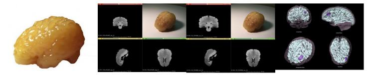
A professional brain phantom. Anatomically correct, made based on the average human brain, performed from realistic materials that mimic human tissues. Phantom is intended for ultrasonography diagnostic (USG), magnetic resonance (MRI) and tomography (CT) training.
