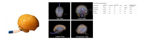
A professional, multipurpose brain phantom. Anatomically correct, made based on the average human brain, built from realistic materials that mimic human tissues. Phantom is intended for ultrasonography diagnostic (USG), magnetic resonance (MRI) and tomography (CT) training.
