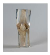
A phantom of the knee joint designed for performing X-ray photography. Has a distal part of the femur, proximal fragment of tibia and fibula bone and patella. The whole is embedded in a special, transparent material, which does not cause image artifacts.
