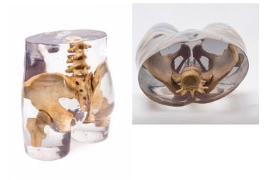
The pelvis of an adult human with the lower lumbar vertebrae and proximal parts of the femurs, embedded in a special, transparent material that does not cause image artifacts. Phantom is designed to take X-ray pictures.
