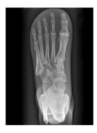
Phantom containing the bones of the foot and distal par of tibia and fibula, intended for performing X-ray images. The bones were embedded in a special,non- transparent material that did not cause image artifacts.
