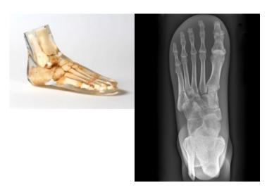
Phantom containing the bones of the foot and distal part of tibia and fibula, intended for performing X-ray photography.
