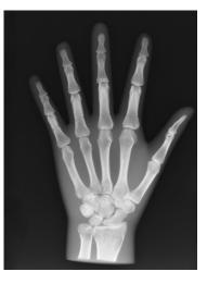
An adult man's hand together with wrist bones and distal fragments of the forearm bone, embedded in a special, transparent material that does not cause image artifacts. Phantom is designed to take X-ray pictures.
