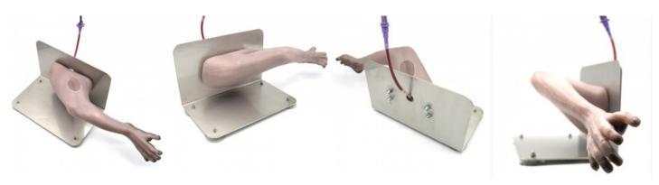
Enables training of injection skills in adult rhesus monkeys. Integrated hip joint allows simulation of handling and fixation of the thigh. A blood draw and injection into a femoral vein can realistically be done on the inside of the thigh. It is also possible to apply venous catheters to the skin-like venous module.
