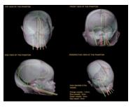
Anatomically correct newborn head phantom. Phantom is designed to imaging the medical flow of blood under the skull. It has been designed based on the average head of a newborn and is made of realistic materials that mimic the soft and hard tissue of appropriate structures for USG, MRI and CT applications.
