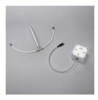
This accessory to permits two Beating Hearts (one with Ancillary) to be powered by a single source of compressed air
