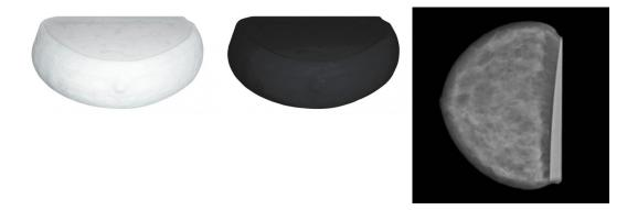
Breast phantom with adipose and glandular tissue. This breast phantom was developed to simulate breast imaging in mammography and tomosynthesis.
