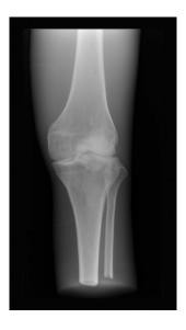
A phantom of the knee joint designed for performing X-ray photography. Has a distal part of the femur, proximal fragment of tibia and fibula bone and patella. The whole is embedded in a special, nontransparent material, which does not cause image artifacts.
