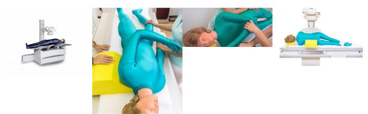
**Life-size X-ray Phantom**. It contains a real human skeleton that allows taking real X-ray images comparable to a real patient. Using a real skeleton allows to visualize even the smallest anatomic details, which is not possible in a plastic skeleton.
