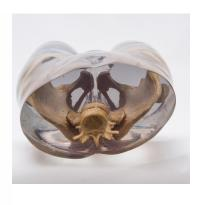
The pelvis of an adult human with the lower lumbar vertebrae and proximal parts of the femurs, embedded in a special, transparent material that does not cause image artifacts. Phantom is designed to take X-ray pictures.
