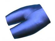
The pelvis of an adult human with the lower lumbar vertebrae and proximal parts of the femurs, embedded in a special, non-transparent material that does not cause image artifacts. Phantom is designed to take X-ray pictures.
