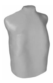
A chest phantom designed for performing X-ray photography. The following bones were embedded in the soft material:
