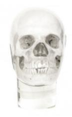
Human skull designed for radiographic examinations, embedded in a special, transparent material that does not cause image artifacts.
