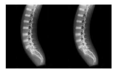
A vertebral column phantom designed for performing X-ray photography. The following bones were embedded in the nontransparent material:
