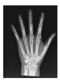
An adult man's hand together with wrist bones and distal fragments of the forearm bone, embedded in a special, non- transparent material that does not cause image artifacts. Phantom is designed to take X-ray pictures.
